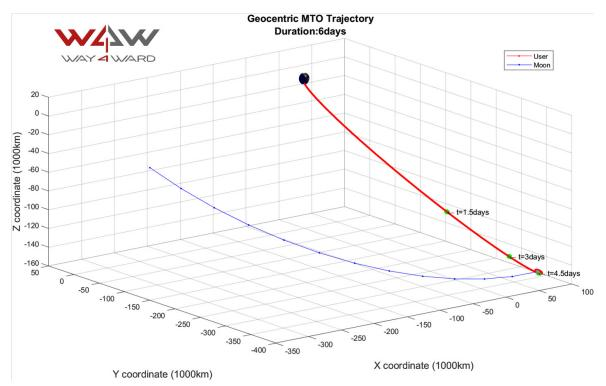
Figure 6: Geocentric Moon Transfer Orbit (MTO) trajectory (duration ~ 6 days)
