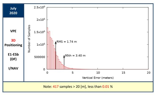
Figure 17: Vertical Positioning Error (VPE) for "Galileo-only" users in July 2020
