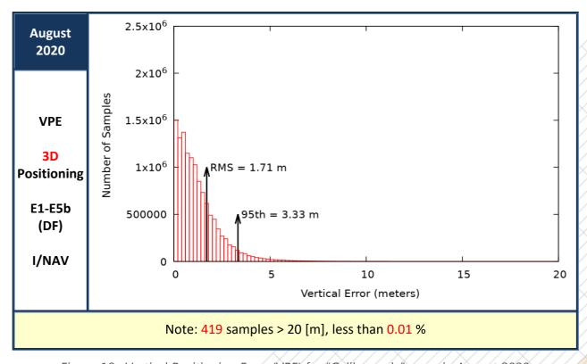
Figure 18: Vertical Positioning Error (VPE) for "Galileo-only" users in August 2020
