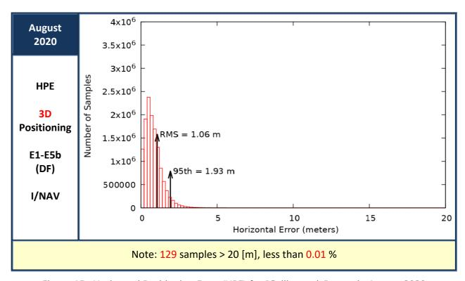
Figure 15: Horizontal Positioning Error (HPE) for "Galileo-only" users in August 2020
