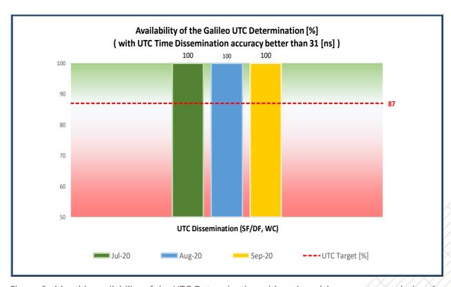
Figure 6 : Monthly availability of the UTC Determination with assigned Accuracy target during the reporting period
