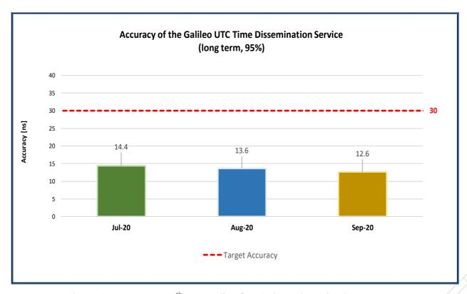
Figure 8 : Long-term 95<sup>th</sup> percentile of UTC Time Dissemination Accuracy
