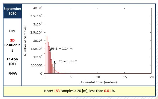
Figure 16: Horizontal Positioning Error (HPE) for "Galileo-only" users in September 2020
