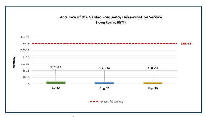
Figure 9 : Long-term 95<sup>th</sup> percentile of UTC Frequency Dissemination Accuracy
