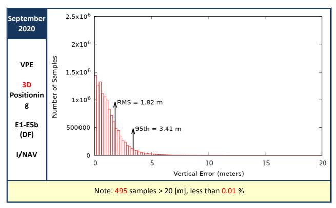
Figure 19: Vertical Positioning Error (VPE) for "Galileo-only" users in September 2020
