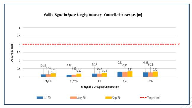
Figure 4 : Monthly Galileo SIS Ranging Accuracy (95<sup>th</sup> percentile) "over all satellites" (constellation average), measured during the reporting period
