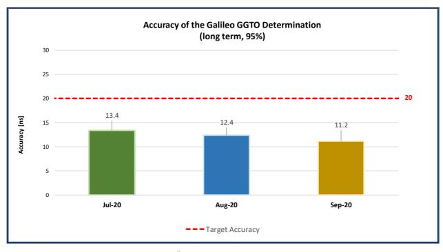
Figure 10: Long-term 95<sup>th</sup> percentile of GGTO Determination Accuracy
