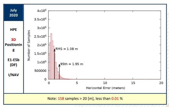
Figure 14: Horizontal Positioning Error (HPE) for "Galileo-only" users in July 2020
