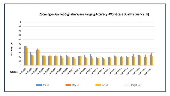
Figure 2 : Monthly Galileo SIS Ranging Accuracy (95<sup>th</sup> percentile) "for any satellite", measured during reporting period for worst-case, Dual-Frequency (DF)
