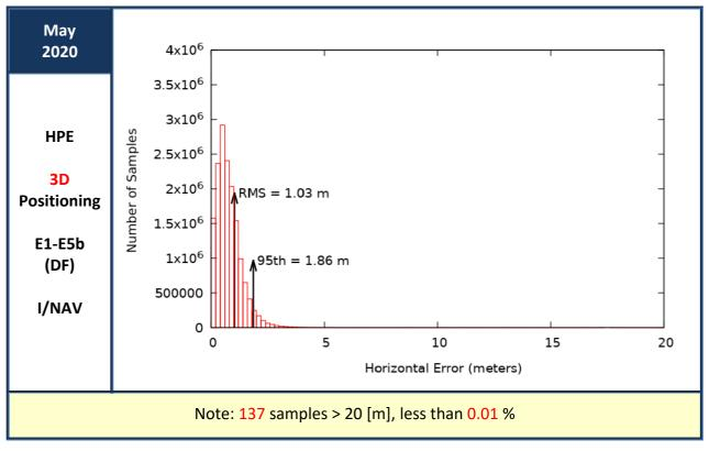
Figure 15 : Horizontal Positioning Error (HPE) for "Galileo-only" users in May 2020
