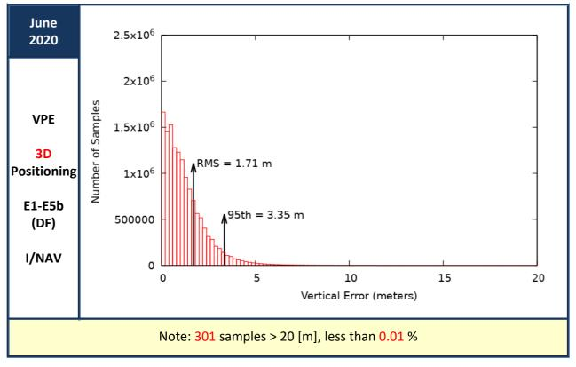
Figure 19 : Vertical Positioning Error (VPE) for "Galileo-only" users in June 2020
