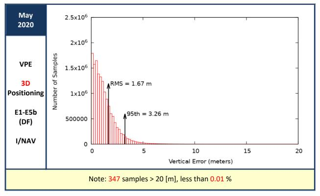
Figure 18 : Vertical Positioning Error (VPE) for "Galileo-only" users in May 2020
