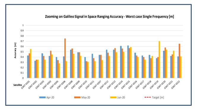
Figure 3 : Monthly Galileo SIS Ranging Accuracy (95<sup>th</sup> percentile) "for any satellite", measured during the reporting period for worst-case, Single-Frequency (SF)
