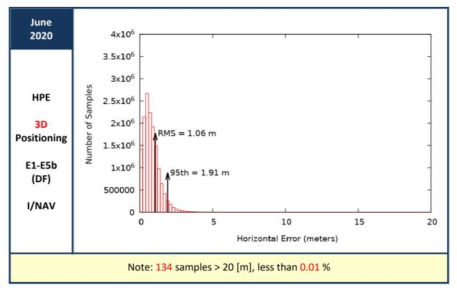
Figure 16 : Horizontal Positioning Error (HPE) for "Galileo-only" users in June 2020
