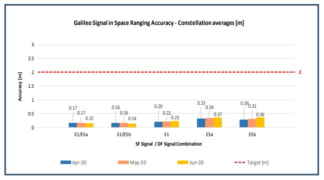
Figure 4 : Monthly Galileo SIS Ranging Accuracy (95<sup>th</sup> percentile) "over all satellites" (constellation average), measured during the reporting period
