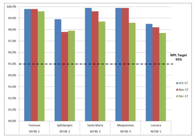
Figure 5: Per Reference Beacon Probability of 5km Accuracy in Multi-Burst
