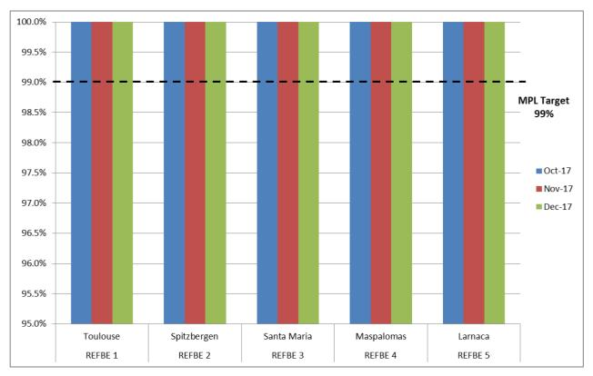
Figure 1: Per Reference Beacon Single Burst Detection Probability
