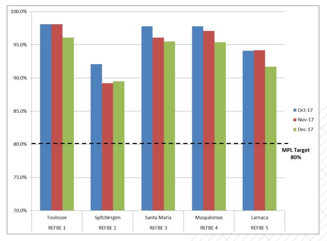
Figure 6: Per Reference Beacon Probability of 2km Accuracy in Multi-Burst
