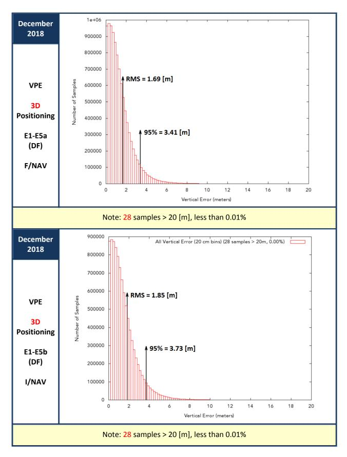
Figure 18: Vertical Positioning Error (VPE) for Galileo only users in December 2018
