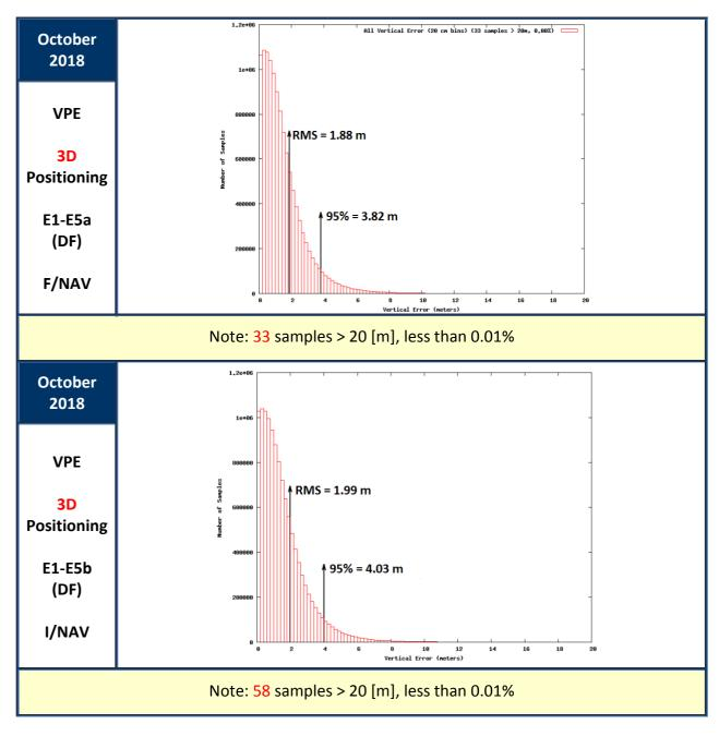
Figure 16: Vertical Positioning Error (VPE) for Galileo only users in October 2018
