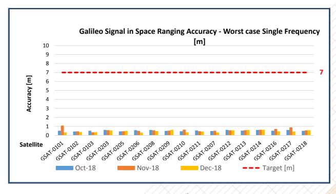
Figure 4: Monthly Galileo SIS Ranging Accuracy (95<sup>th</sup> percentile) "for any satellite", measured during the reporting period for worst-case, Single-Frequency (SF)
