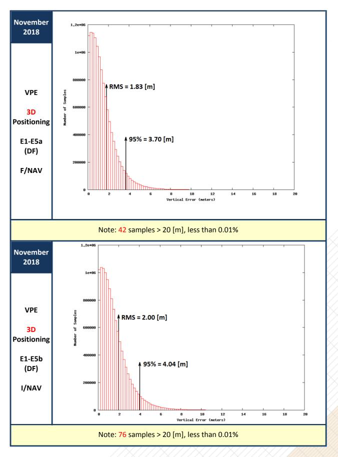
Figure 17: Vertical Positioning Error (VPE) for Galileo only users in November 2018
