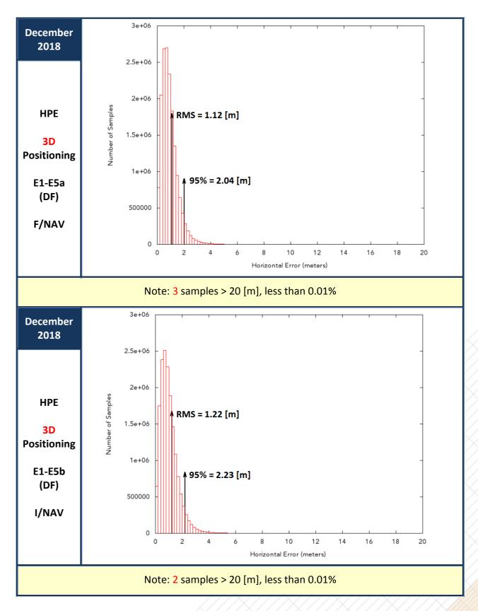
Figure 15: Horizontal Positioning Error (HPE) for "Galileo-only" users in December 2018
