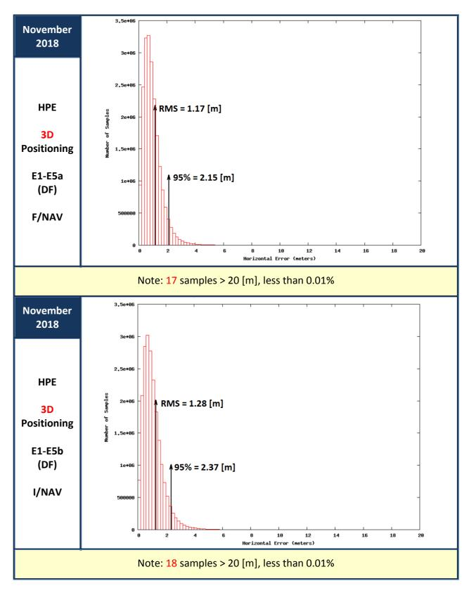
Figure 14: Horizontal Positioning Error (HPE) for "Galileo-only" users in November 2018
