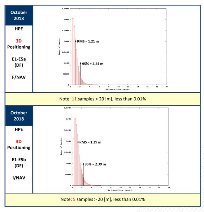
Figure 13: Horizontal Positioning Error (HPE) for "Galileo-only" users in October 2018
