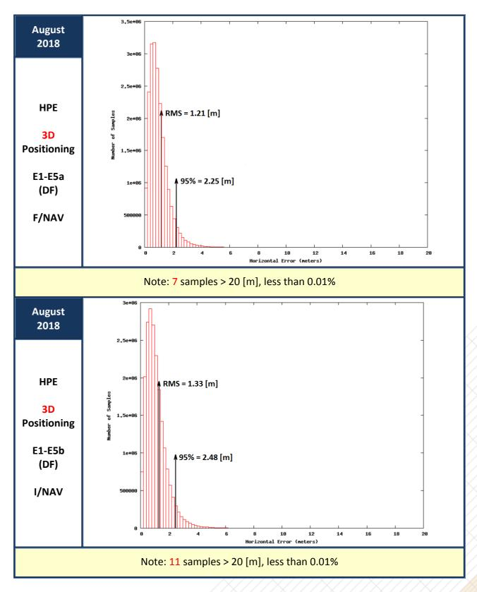
Figure 14: Horizontal Positioning Error (HPE) for "Galileo-only" users in August 2018
