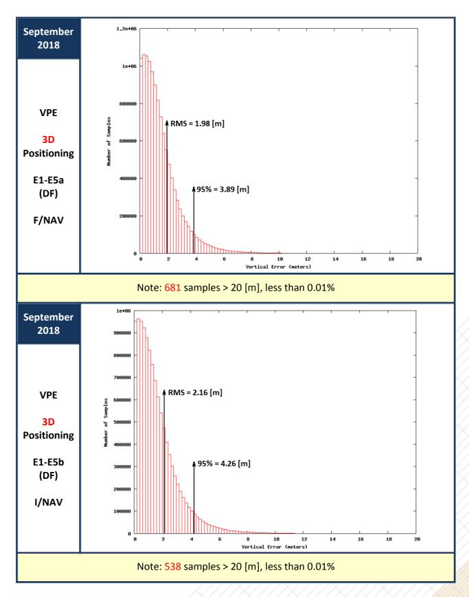
Figure 18: Vertical Positioning Error (VPE) for Galileo only users in September 2018
