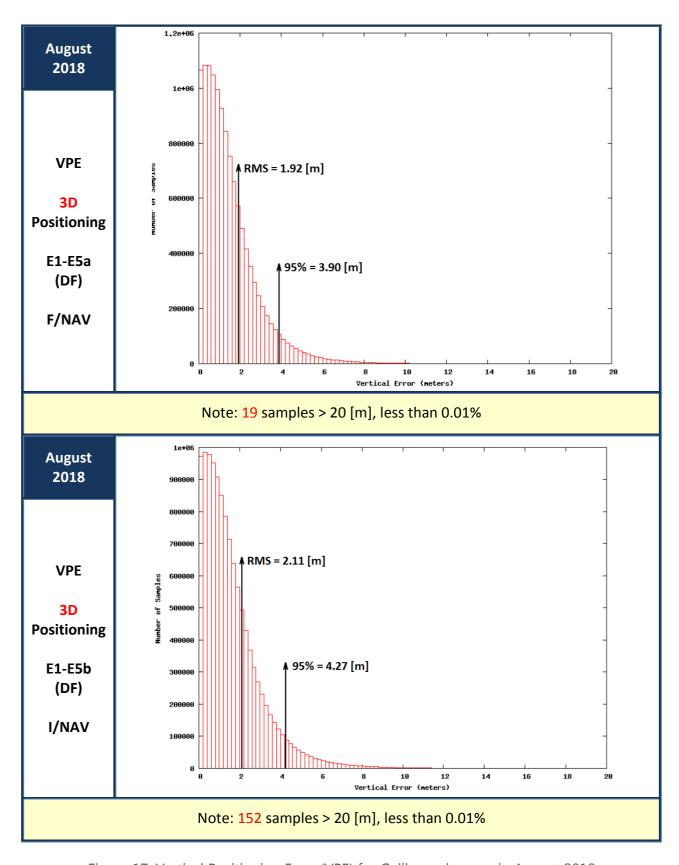
Figure 17: Vertical Positioning Error (VPE) for Galileo only users in August 2018
