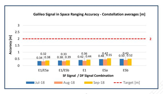
Figure 5: Monthly Galileo SIS Ranging Accuracy (95<sup>th</sup> percentile) "over all satellites" (constellation average), measured during the reporting period
