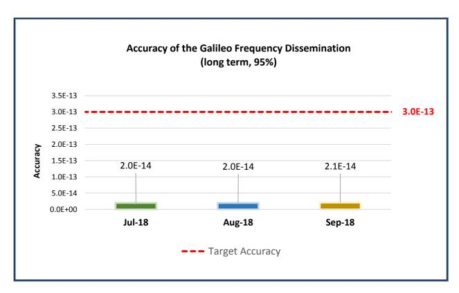
Figure 10: Long-term 95<sup>th</sup> percentile of UTC Frequency Dissemination Accuracy
