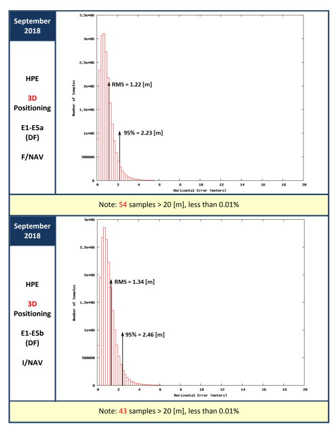
Figure 15: Horizontal Positioning Error (HPE) for "Galileo-only" users in September 2018
