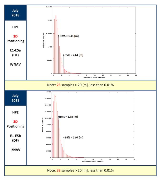
Figure 13: Horizontal Positioning Error (HPE) for "Galileo-only" users in July 2018
