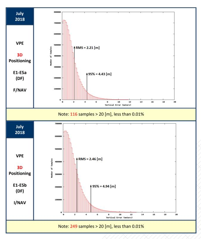
Figure 16: Vertical Positioning Error (VPE) for Galileo only users in July 2018
