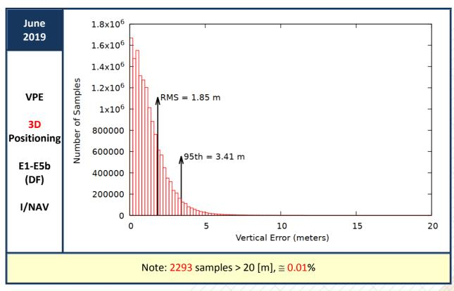
Figure 20: Vertical Positioning Error (VPE) for "Galileo-only" users in June 2019
