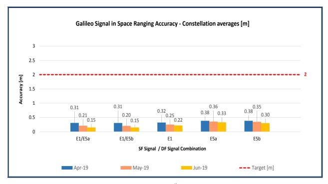
Figure 5: Monthly Galileo SIS Ranging Accuracy (95<sup>th</sup> percentile) "over all satellites" (constellation average), measured during the reporting period
