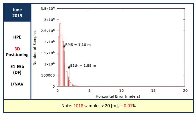
Figure 17: Horizontal Positioning Error (HPE) for "Galileo-only" users in June 2019
