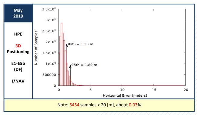
Figure 16: Horizontal Positioning Error (HPE) for "Galileo-only" users in May 2019
