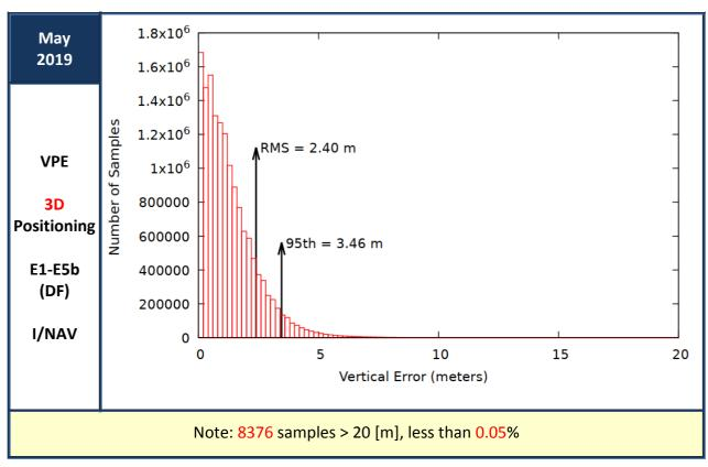
Figure 19: Vertical Positioning Error (VPE) for "Galileo-only" users in May 2019
