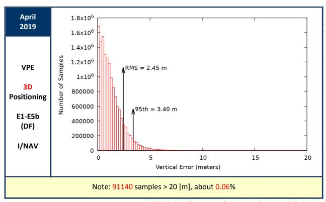
Figure 18: Vertical Positioning Error (VPE) for "Galileo-only" users in April 2019
