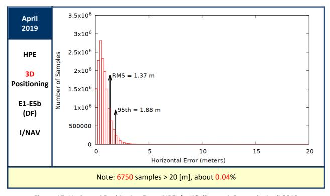
Figure 15: Horizontal Positioning Error (HPE) for "Galileo-only" users in April 2019
