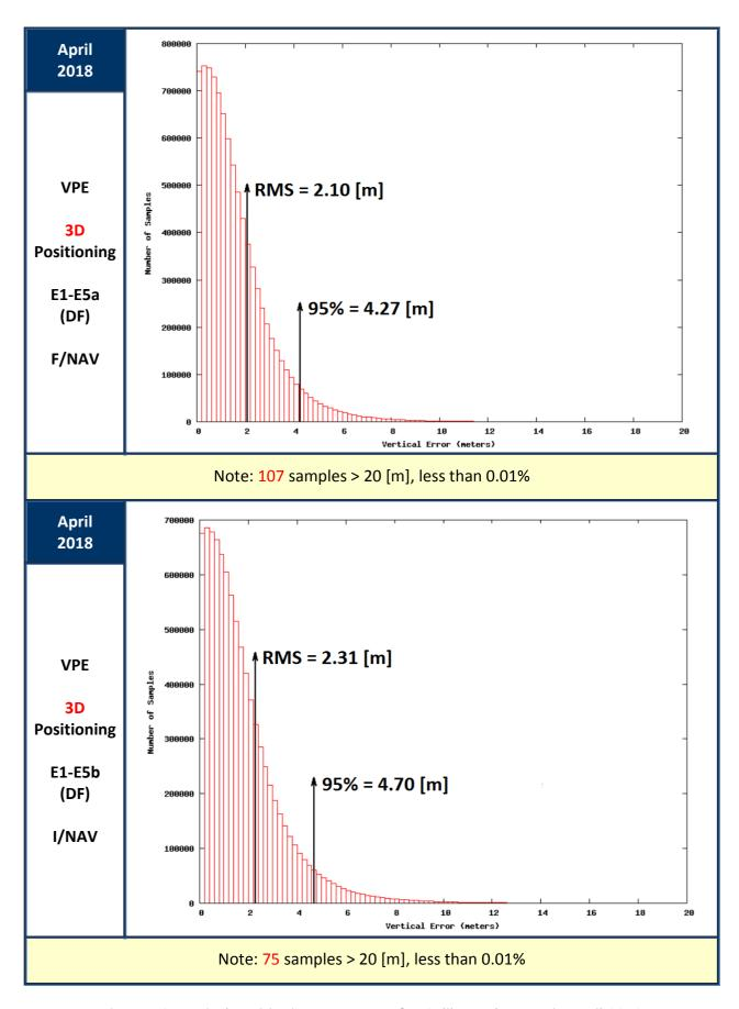
Figure 16: Vertical Positioning Error (VPE) for Galileo only users in April 2018
