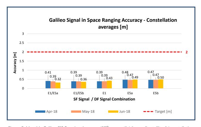
Figure 5: Monthly Galileo SIS Ranging Accuracy (95<sup>th</sup> percentile) "over all satellites" (constellation average), measured during the reporting period
