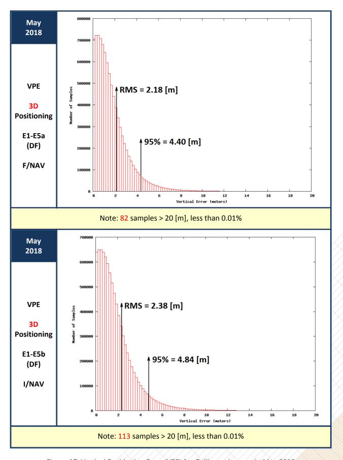
Figure 17: Vertical Positioning Error (VPE) for Galileo only users in May 2018
