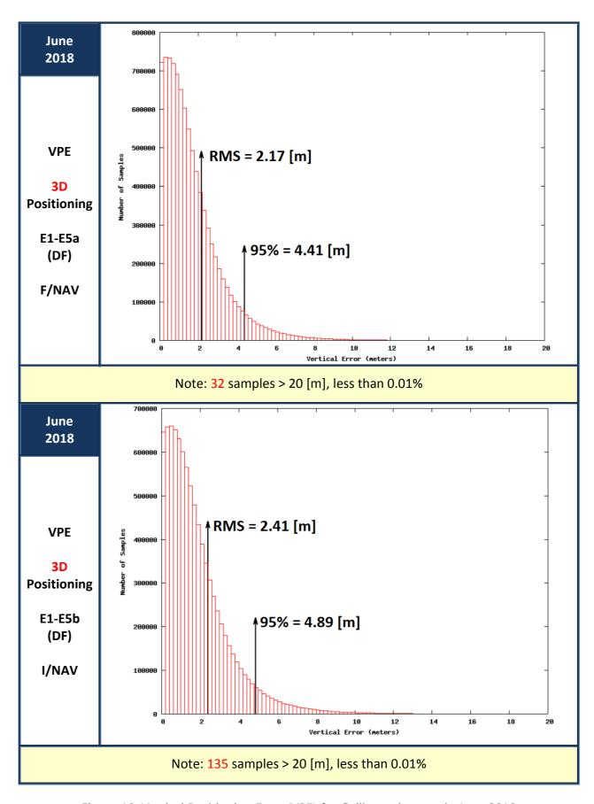
Figure 18: Vertical Positioning Error (VPE) for Galileo only users in June 2018
