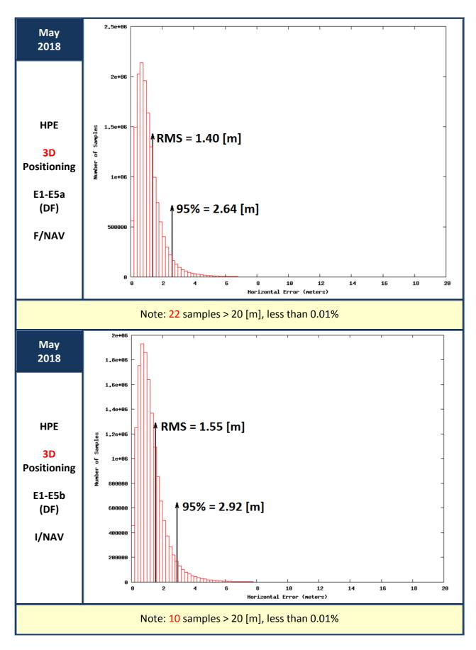
Figure 14: Horizontal Positioning Error (HPE) for "Galileo-only" users in May 2018
