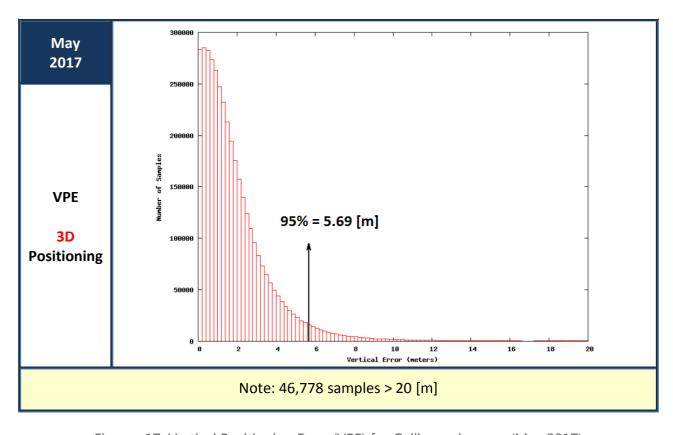
Figures 17: Vertical Positioning Error (VPE) for Galileo only users (May 2017)
