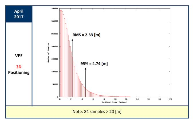
Figures 16: Vertical Positioning Error (VPE) for Galileo only users (April 2017)
