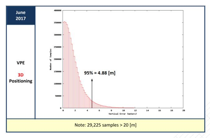
Figures 18: Vertical Positioning Error (VPE) for Galileo only users (June 2017)
