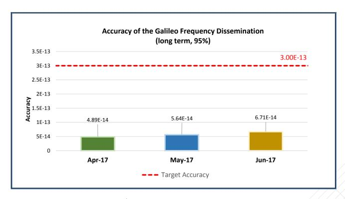
Figure 10: Long-term 95<sup>th</sup> percentile of UTC Frequency Dissemination Accuracy
