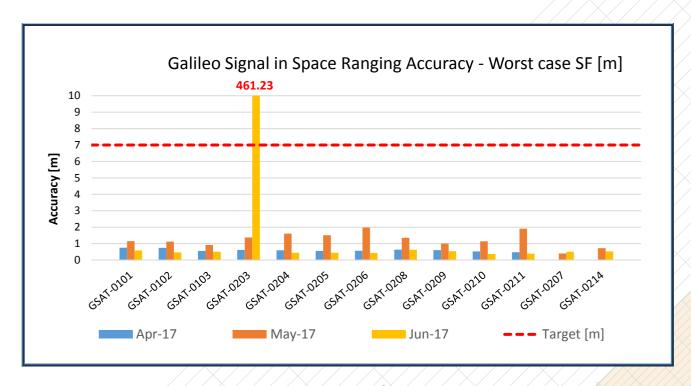
Figure 4: Monthly Galileo SIS Ranging Accuracy (95<sup>th</sup> percentile) "for any satellite", measured during reporting period for worst-case, Single-Frequency (SF)
