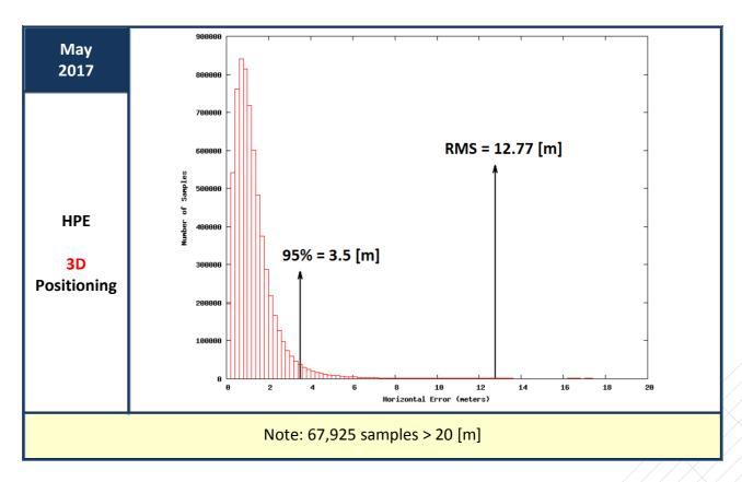
Figure 14: Horizontal Positioning Error (HPE) for "Galileo-only" users (May 2017)
