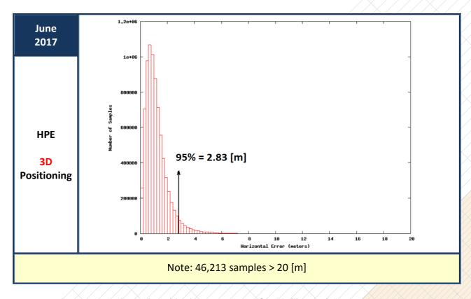
Figure 15: Horizontal Positioning Error (HPE) for "Galileo-only" users (June 2017)
