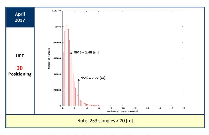
Figure 13: Horizontal Positioning Error (HPE) for "Galileo-only" users (April 2017)
