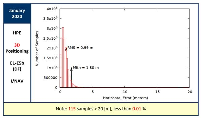
Figure 14: Horizontal Positioning Error (HPE) for "Galileo-only" users in January 2020
