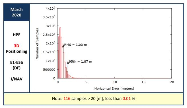
Figure 16: Horizontal Positioning Error (HPE) for "Galileo-only" users in March 2020
