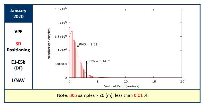
Figure 17: Vertical Positioning Error (VPE) for "Galileo-only" users in January 2020
