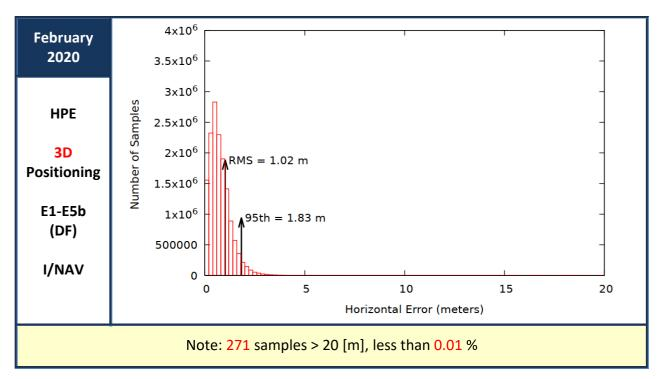
Figure 15: Horizontal Positioning Error (HPE) for "Galileo-only" users in February 2020
