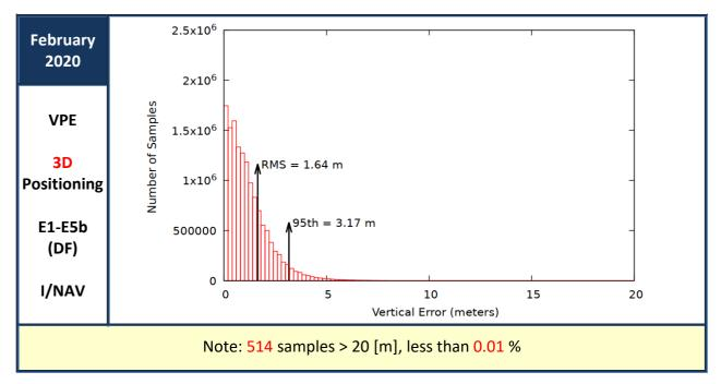
Figure 18: Vertical Positioning Error (VPE) for "Galileo-only" users in February 2020
