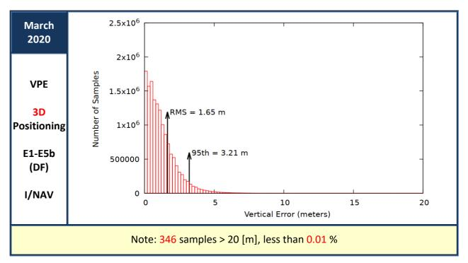
Figure 19: Vertical Positioning Error (VPE) for "Galileo-only" users in March 2020
