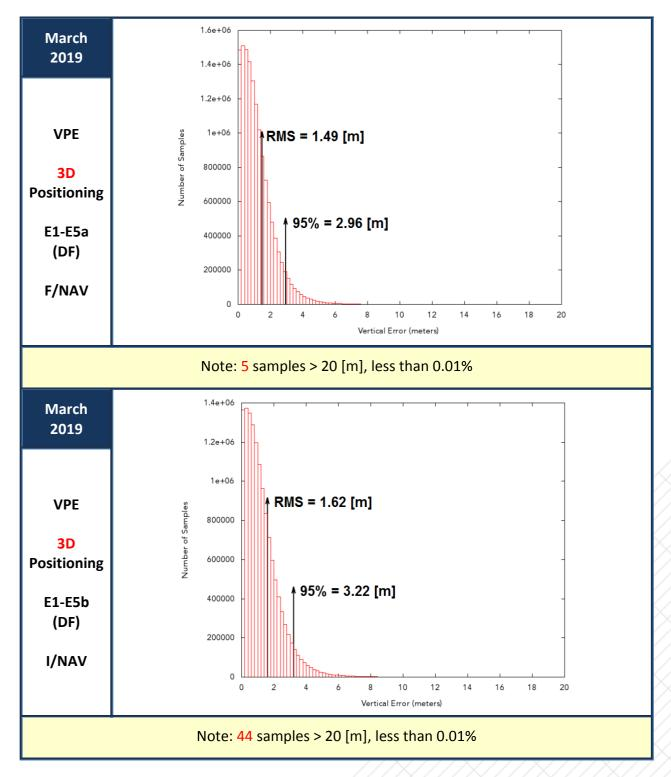
Figure 18: Vertical Positioning Error (VPE) for "Galileo-only" users in March 2019
