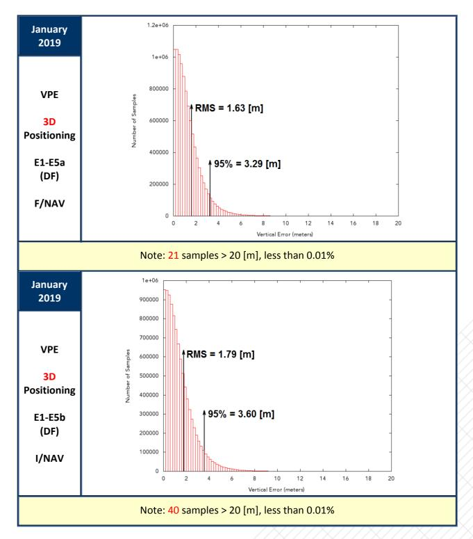
Figure 16: Vertical Positioning Error (VPE) for "Galileo-only" users in January 2019
