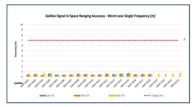
Figure 4: Monthly Galileo SIS Ranging Accuracy (95<sup>th</sup> percentile) "for any satellite", measured during the reporting period for worst-case, Single-Frequency (SF)
