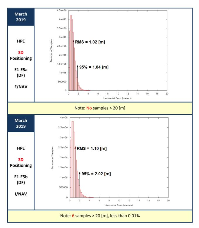
Figure 15: Horizontal Positioning Error (HPE) for "Galileo-only" users in March 2019
