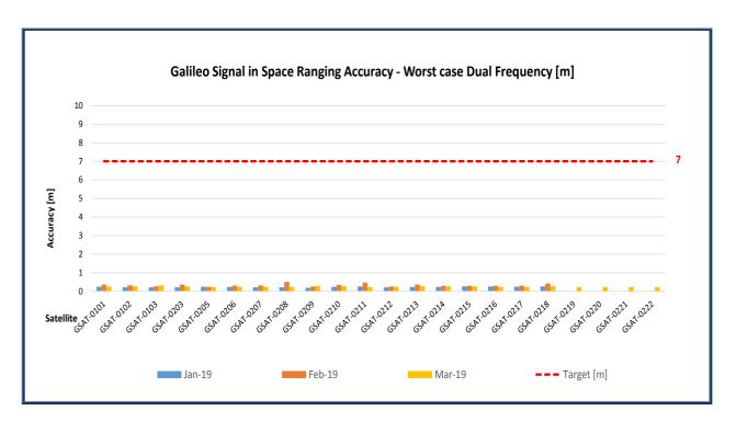
Figure 3: Monthly Galileo SIS Ranging Accuracy (95<sup>th</sup> percentile) "for any satellite", measured during reporting period for worst-case, Dual-Frequency (DF)
