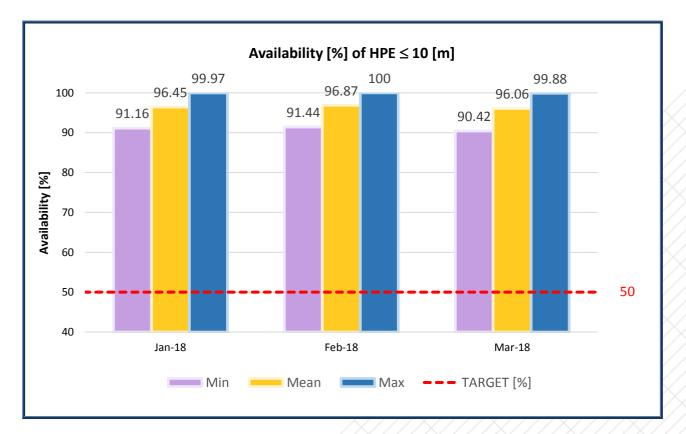
Figure 12: Availability of the Galileo Horizontal Positioning Service with Accuracy  $\leq$  10 [m]
