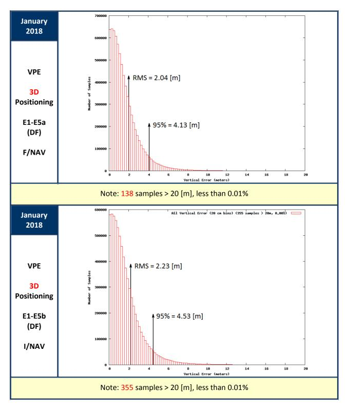
Figure 16: Vertical Positioning Error (VPE) for Galileo only users in January 2018
