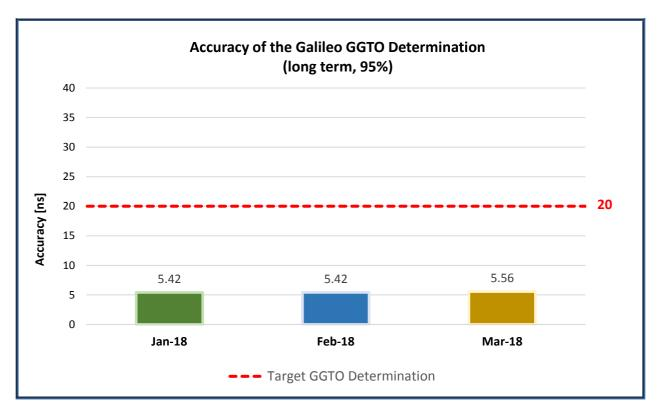
Figure 9: Long-term 95<sup>th</sup> percentile of GGTO Determination Accuracy
