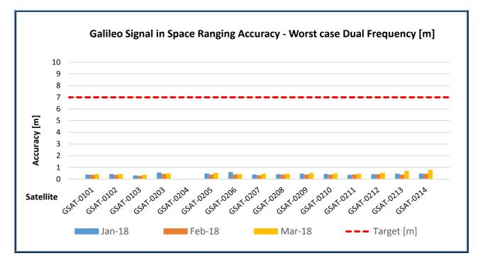
Figure 3: Monthly Galileo SIS Ranging Accuracy (95<sup>th</sup> percentile) "for any satellite", measured during reporting period for worst-case, Dual-Frequency (DF)
