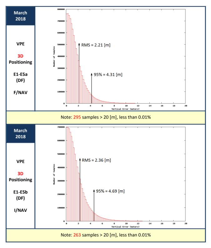
Figure 18: Vertical Positioning Error (VPE) for Galileo only users in March 2018
