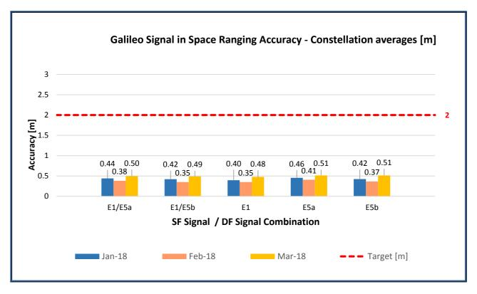
Figure 5: Monthly Galileo SIS Ranging Accuracy (95<sup>th</sup> percentile) "over all satellites" (constellation average), measured during the reporting period
