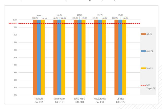
Figure 6: Per Reference Beacon Valid Message Detection Probability (in %)
