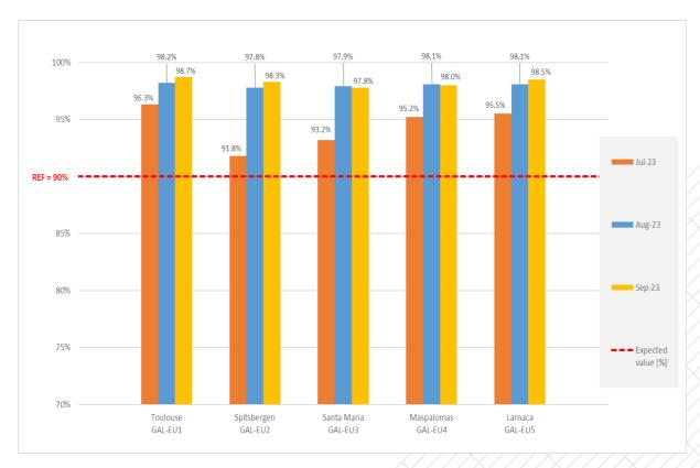
Figure 12: Per Reference Beacon Probability of two-kilometre Accuracy in Multi-Burst (in %)
