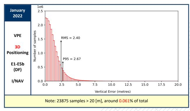
Figure 22: Vertical Positioning Error (VPE) for "Galileo-only" users in January 2022
