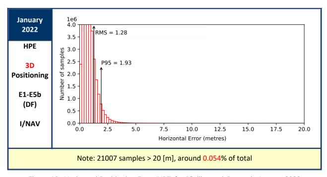
Figure 19: Horizontal Positioning Error (HPE) for "Galileo-only" users in January 2022
