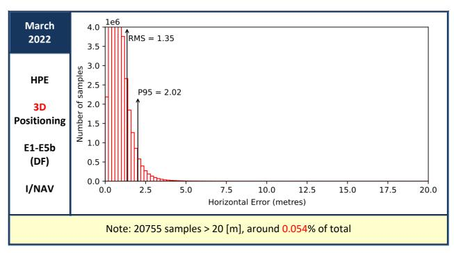
Figure 21: Horizontal Positioning Error (HPE) for "Galileo-only" users in March 2022
