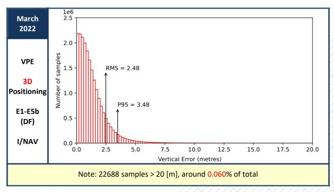
Figure 24: Vertical Positioning Error (VPE) for "Galileo-only" users in March 2022
