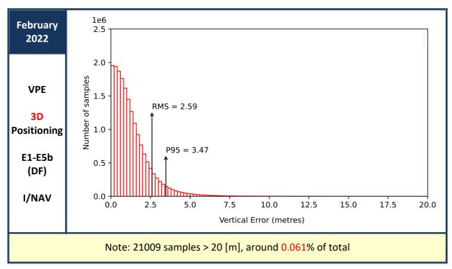
Figure 23: Vertical Positioning Error (VPE) for "Galileo-only" users in February 2022
